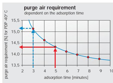
with 5 minutes adsorption, gives 12 load alternations per hour. The customary 6 minute cycle of market competitors, with 3 minutes adsorption, gives 20 load alternations per hour and thus necessarily requires 5.6% more regenerating air. ZANDER 10 minute cycle operation implies energy saving and less wear.
